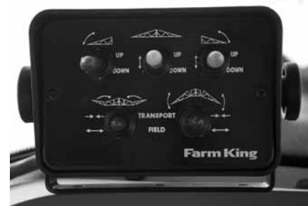
Boom Control Box
