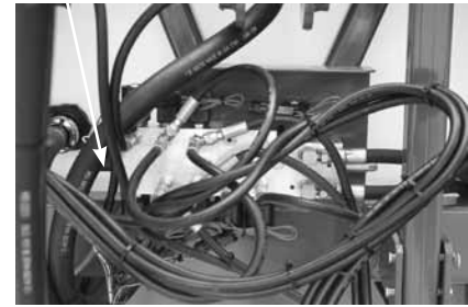
Directional Stack Hydraulic Controller closed center hydraulic system set up, rear view
