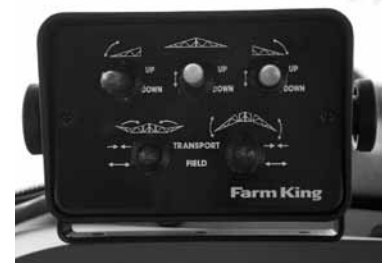
Boom Control Box
