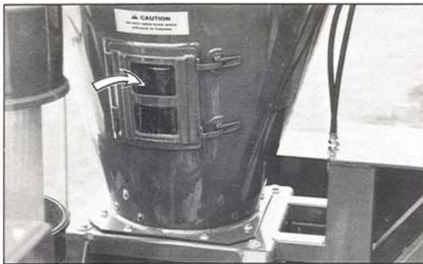
Figure 18 Grain level receiver tank
