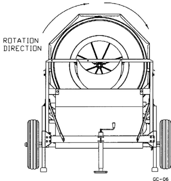
The jack is used both to hook up the cleaner for transport and to adjust the slope of the cleaner.
